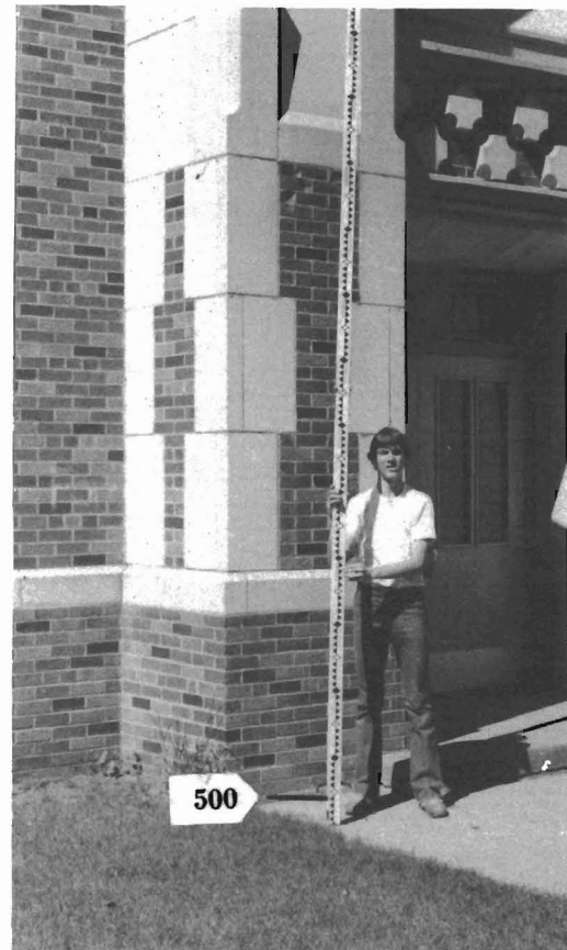
Figure 36. Expected level of the 500-year flood at South Junior High School in Grand Forks. The 100-year flood should not cause serious problems at this point.
