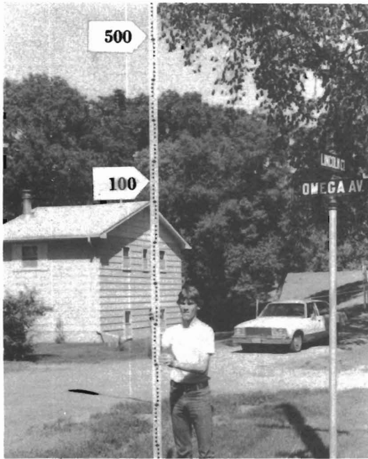
Figure 39. Expected flood heights at the corner of Omega Avenue and Lincoln Court in Grand Forks. This area is protected by a dike and it should be possible to withstand a 100-year flood. It is doubtful that the area could be protected during a 500-year flood.
