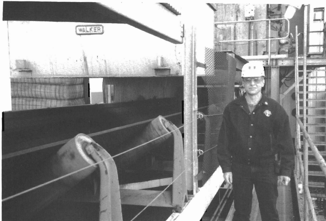
Figure 13. Dennis James (geologist at Falkirk Mine) stands next to a large magnet suspended over the coal conveyor at the Falkirk Mine. The magnet typically removes crushing teeth and parts of dozer blades which occasionally get mixed in with the coal during mining.
