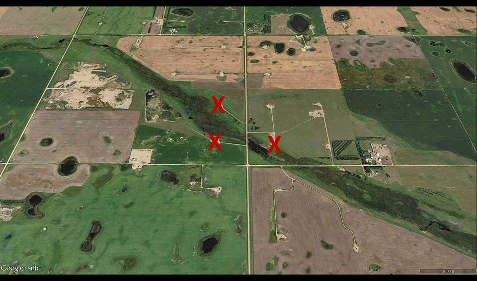
Under today's rules, these locations (X) would require a closed mud system due to a high watertable and near surface sand and gravel deposits.
