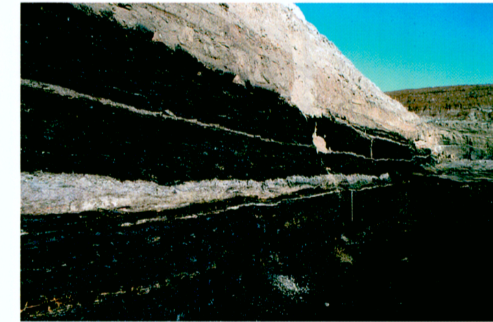
Figure 7. A seven-foot thick seam of leonardite (weathered lignite) exposed in the minefield of GeoResource's pit at Williston. Although lignite and leonardite look similar in outcrop, leonardite is characteristically very soft and powdery.
