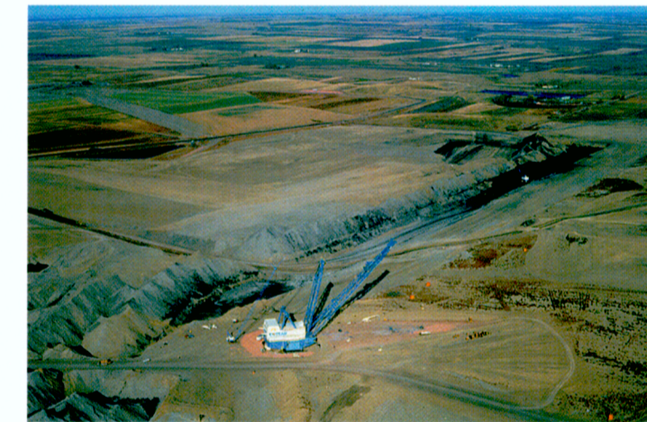
Figure 3. A dragline undergoing maintenance adjacent to an active pit at Coteau's Freedom Mine north of Beulah. View looking northeast. The Beulah-Zap bed has been removed from the west end of the pit and is in the process of being removed from the east end of the pit with a loader.
