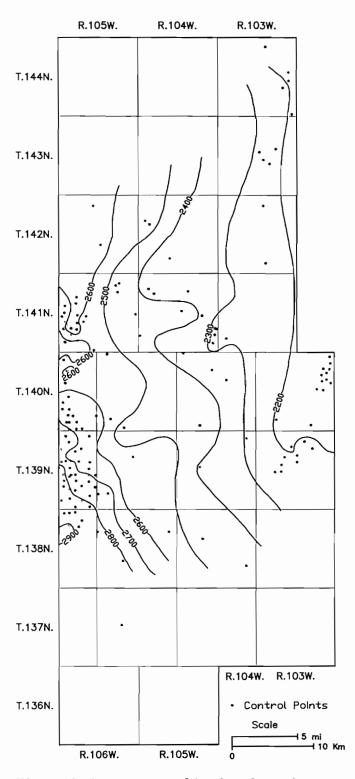
Figure 12. Contour map of the elevation at the top of the Harmon coal in Golden Valley County.
