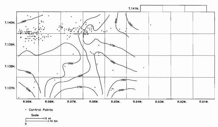
Figure 38. Contour map of the elevation at the top of the Hansen coal in Stark County.
