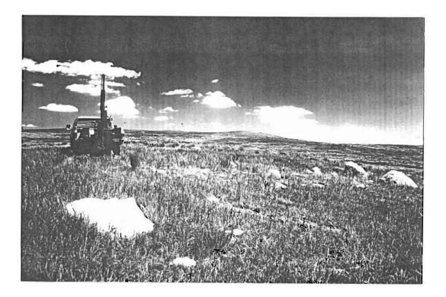
Figure 3. Truck-mounted Giddings soil probe used during this project. The truck is pictured north of Bismarck (T139N, R80W, section 18 nwswse).
