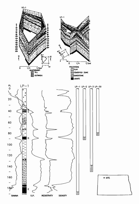
Figure 6. Fence diagram and a monitoring well nest at the Black Slough Field, Burke County, North Dakota.
