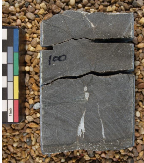
Figure 53. Core photo of calcite filled fractures in Lithofacies 3 in the Sanish Field. This core is from the Deadwood Canyon Ranch #43-28H (NESE Sec. 28, T154N, R92W) and was taken at a depth of 10,100 ft MD.
