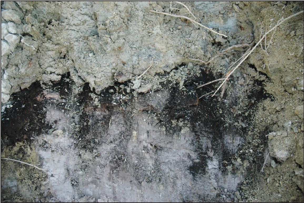
Figure 6. An example of a powder lignite (powder coal or pcoal in the measured sections), sample 55-7.
