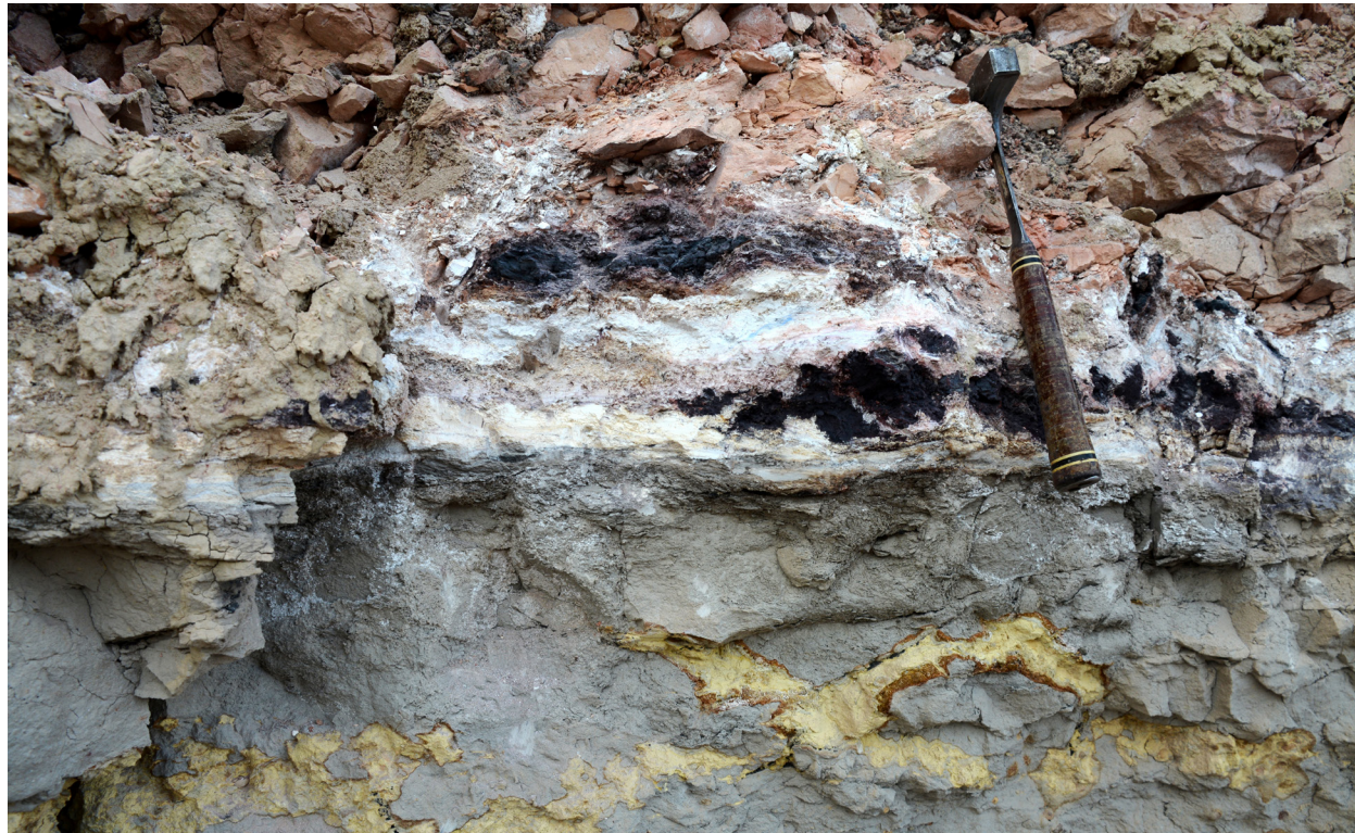
Figure 18. Chunks of clinker within a 7-9 inch ash layer. Note the sharp contact between the ash and the unburned mudstone below (at the base of the rock hammer).
