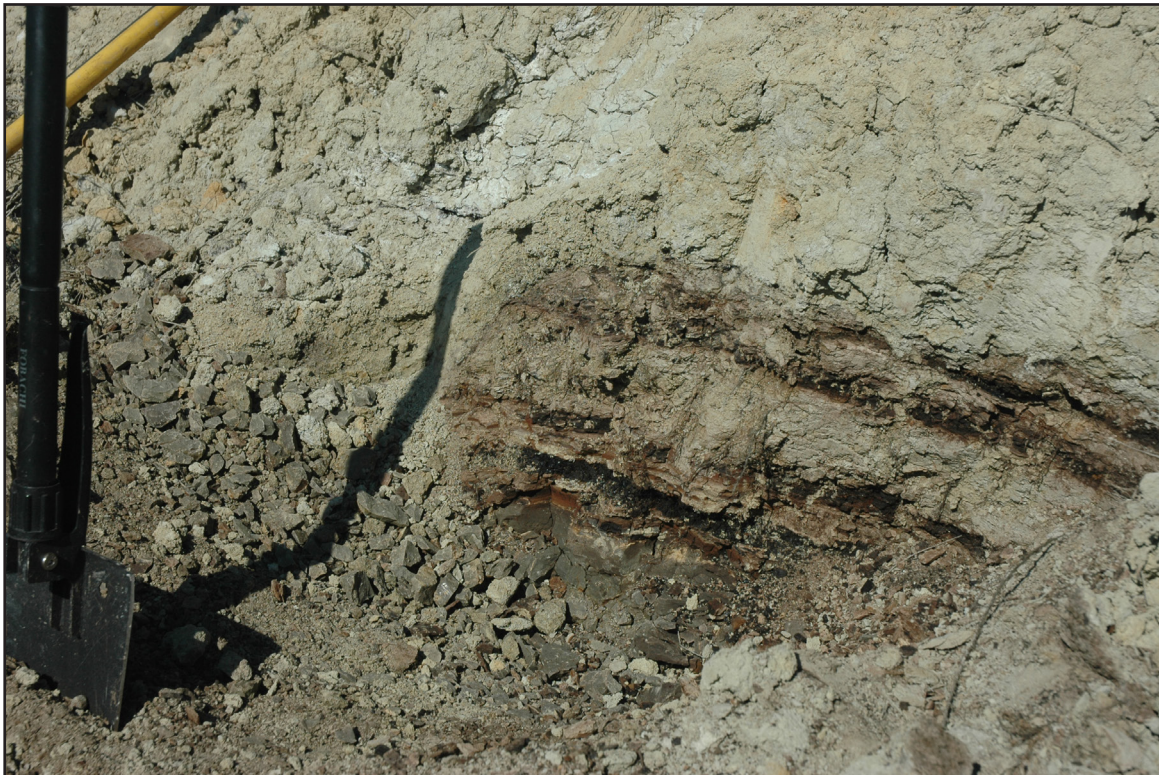
Figure 8. Lenses of lignite within a carbonaceous mudstone (coal lenses in mudstone or clmdst in the measured sections), samples 9A and 9B.
