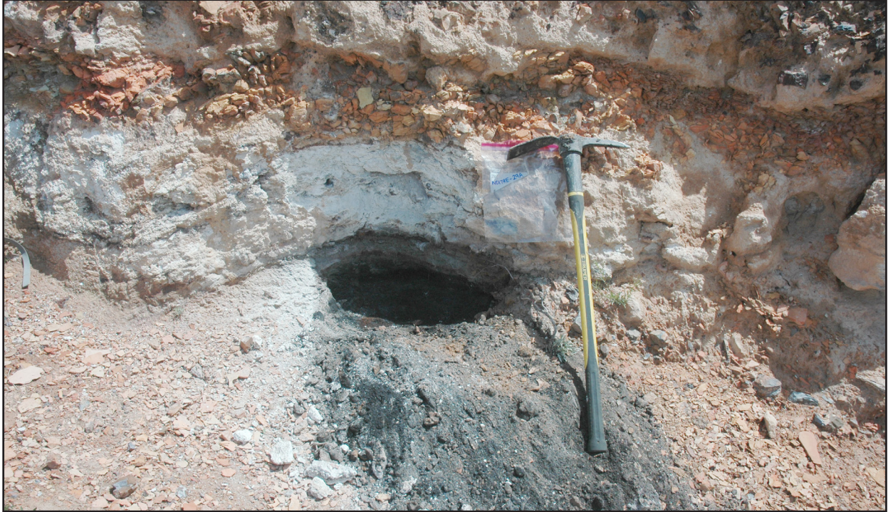
Figure 17. A pit dug beneath a prominent layer of coal ash to reach the contact between ash and the unburned Harmon bed at measured section 53.
