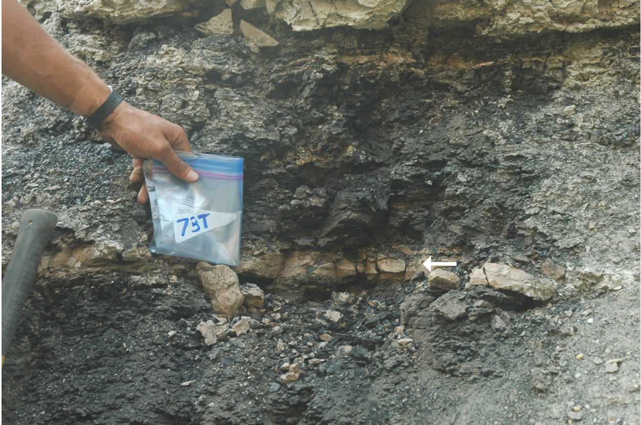
Figure 20. Potential tonstein (arrow) in the upper part of the Hanson bed at measured section no. 73 (sample 73T).
