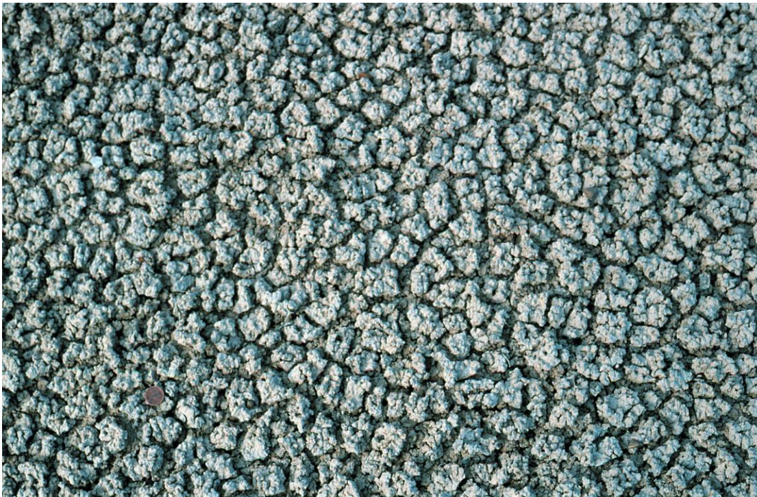
▲ Figure 11. Popcorn texture of the surface of a bentonite layer resulting from the shrinking and expanding of the swelling clays as they alternately hydrate and dehydrate. A penny in the lower left for scale.
