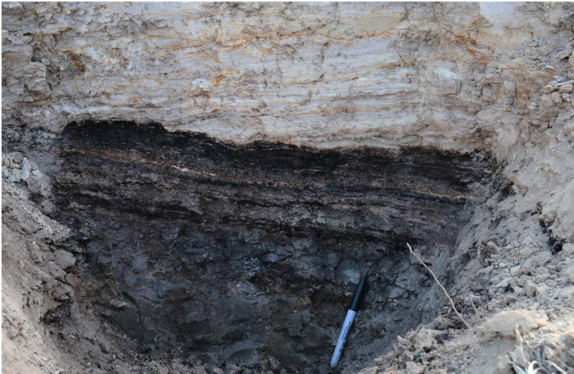
▲ Figure 9. Sample B, measured section no. 2, was taken from the top two inches (5.1 cm) of this one-foot (0.3 m) thick organic-rich bed. As is typical of many of these thin carbonaceous beds, it consists of a mixture of thin lignite layers and even thinner lignite stringers. This bed is overlain by silty mudstone.
