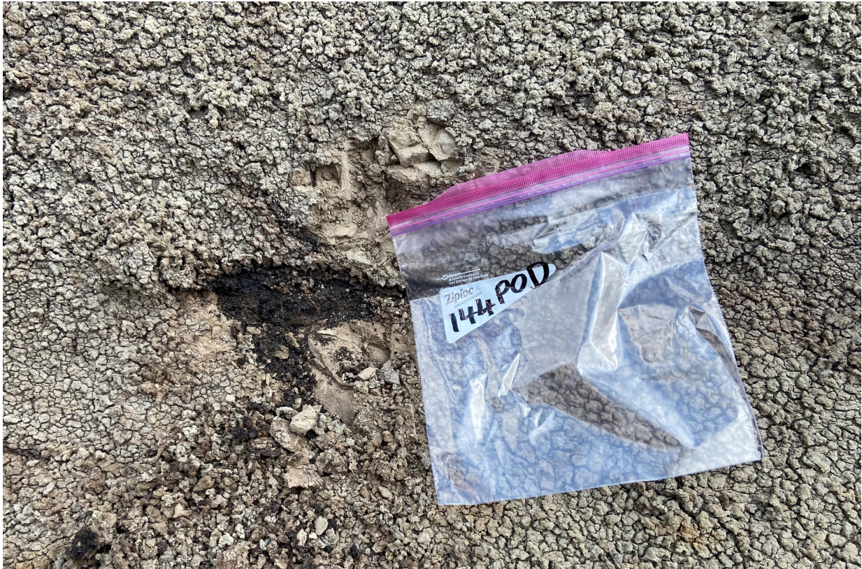
▲ Figure 17. Sample 144(pod), a lens of coal in bentonitic mudstone containing 724 ppm of germanium.
