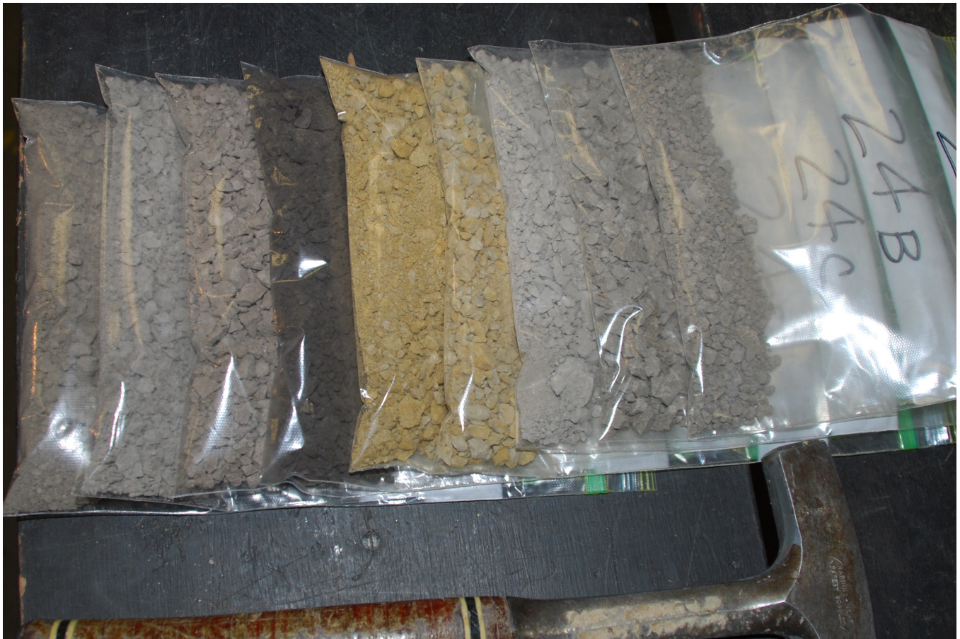
Figure 6. Samples 24a-24i prior to submittal to NDSU. Sample 24a was taken from the top of the Bear Den Member (far right) and Sample 24i was taken from just below the Bear Den Member in the Sentinel Butte Formation (far left). Samples were lightly crushed before they were submitted to the laboratory.
