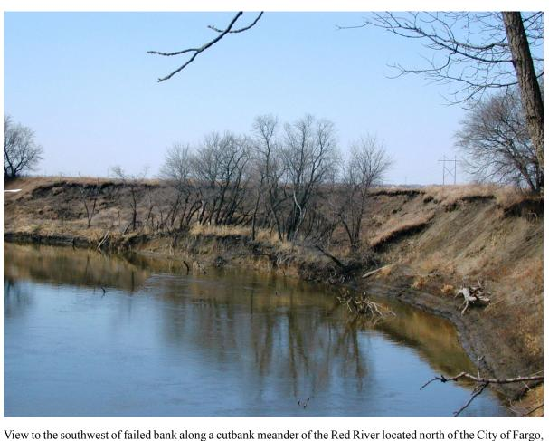
North Dakota. Note the presence of a well defined failure scarp and coherent vegetated slump mass with subvertically orientated trees. The upper Sherack Formation sediments are visible along the cutbank.
