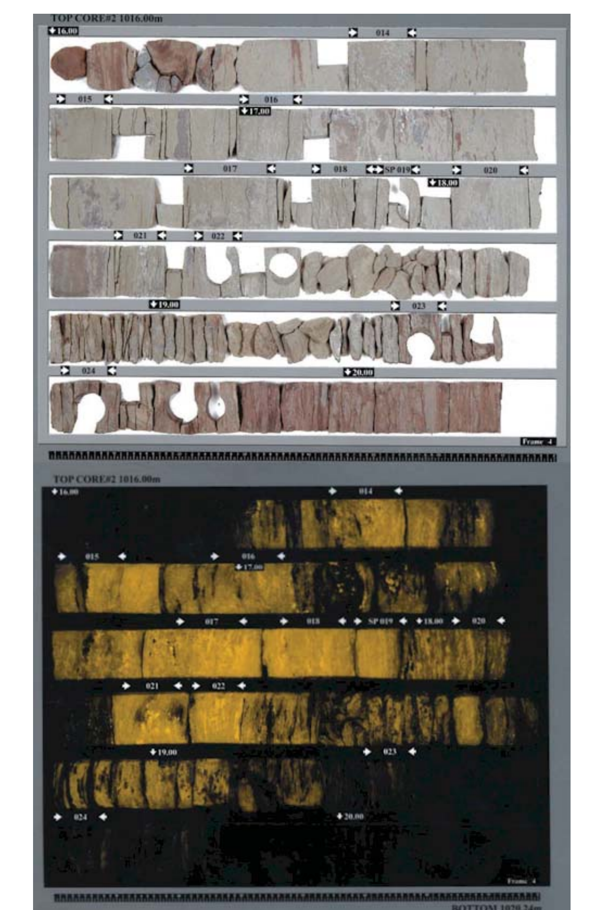
Example of the producing Lower Amaranth, Spearfish equivalent section from Pierson field in Manitoba, Canada. Core photographs are displayed to the right. Porosities increase with the lighter color and are associated with the sandier, cleaner gamma ray sections (Fulton-Regula, 2011). Reservoir issues and best completion and production practices for the Manitoba fields are listed above. XRD data prepared for Molopo Energy Canada, Inc by Agat Laboratories.
