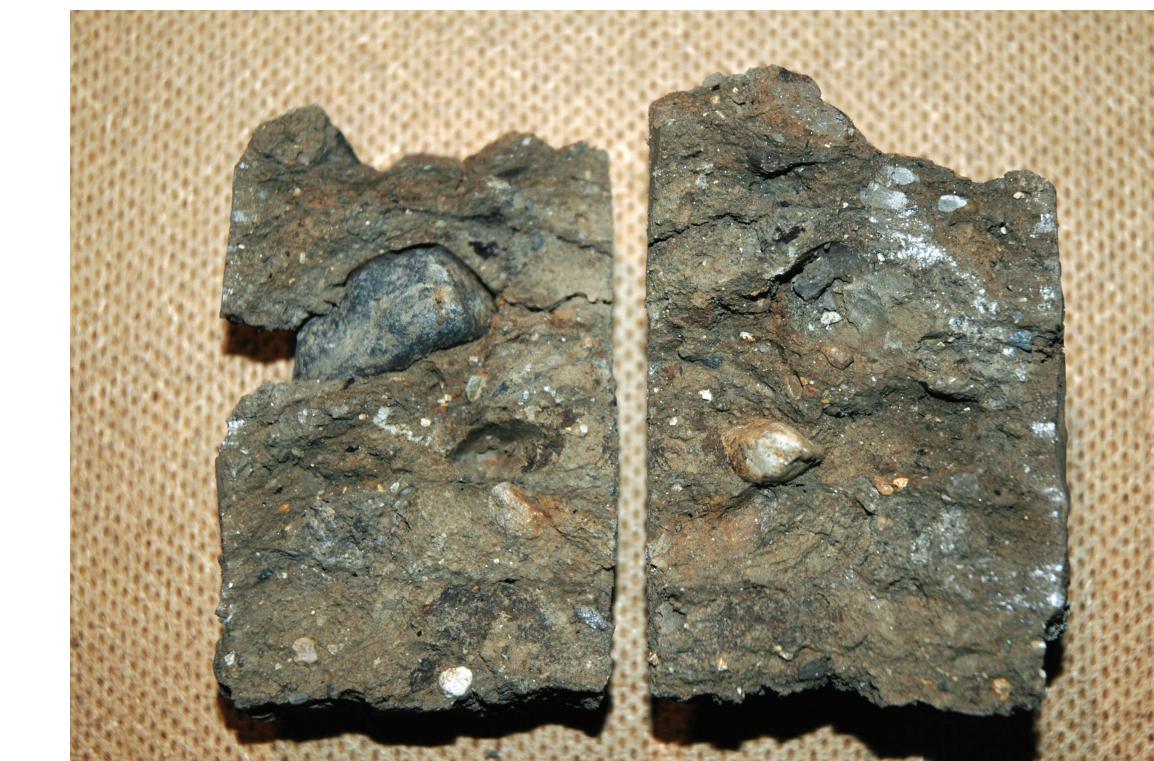
Figure 9. Till from core ND05-012. Depth - 4 m. This material lies directly below the zone tentatively identified as a buried A horizon.
