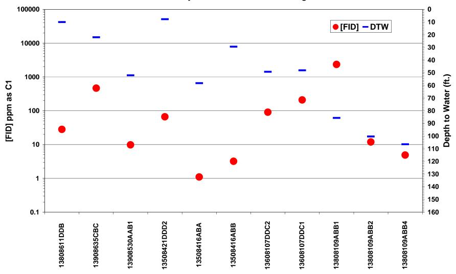
Figure 23. Shallow gas field screening results in Morton County. FID response [FID] in ppm as C1 plotted on the logarithmic scale on the primary y-axis. Depth to water measurements are plotted on the secondary y-axis.
