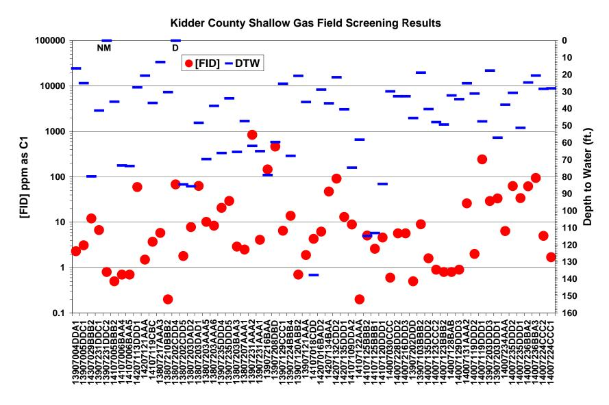
Figure 18. Shallow gas field screening results in Kidder County. FID response [FID] in ppm as C1 plotted on the logarithmic scale on the primary y-axis. Depth to water measurements are plotted on the secondary y-axis. Wells where a water level was not measured (NM) or were dry (DRY) are highlighted.
