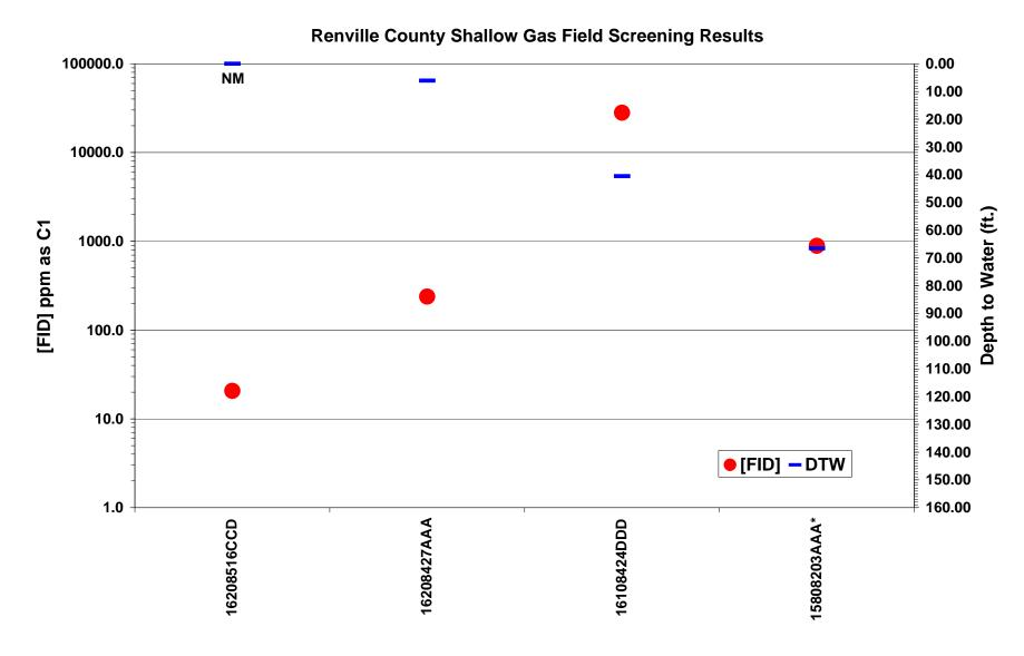
Figure 12. Shallow gas field screening results in Renville County. FID response [FID] in ppm as C1 is plotted on the logarithmic scale on the primary y-axis. Depth to water measurements are plotted on the secondary y-axis. \*Collected on June 26, 2007.
