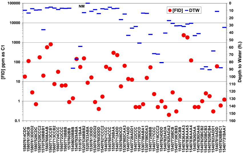
Figure 20. Shallow gas field screening results in McHenry County. FID response [FID] in ppm as C1 plotted on the logarithmic scale on the primary y-axis. Depth to water measurements are plotted on the secondary y-axis.
