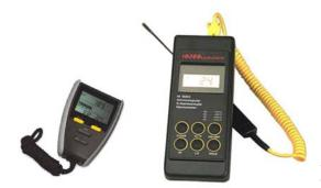
Figure 5. Field instrumentation used for the collection of atmospheric pressure and temperature.
