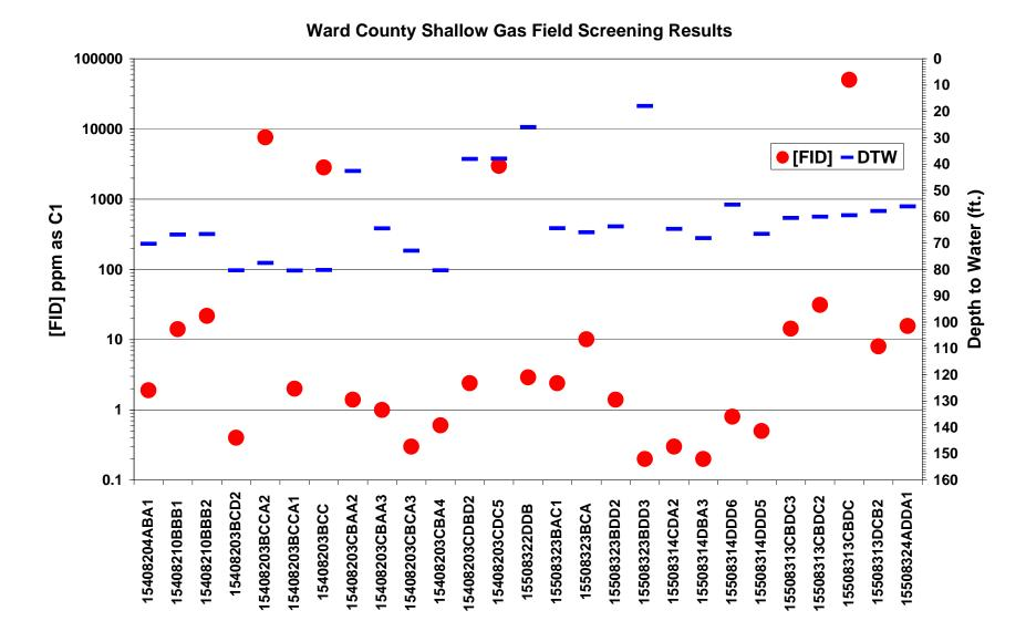
Figure 19. Shallow gas field screening results in Ward County. FID response [FID] in ppm as C1 plotted on the logarithmic scale on the primary y-axis. Depth to water measurements are plotted on the secondary y-axis.
