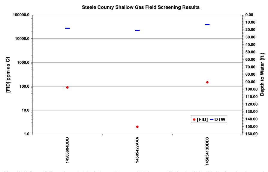
Figure 10. Shallow gas field screening results in Steele County. FID response [FID] in ppm as C1 is plotted on the logarithmic scale on the primary y-axis. Depth to water measurements are plotted on the secondary y-axis.
