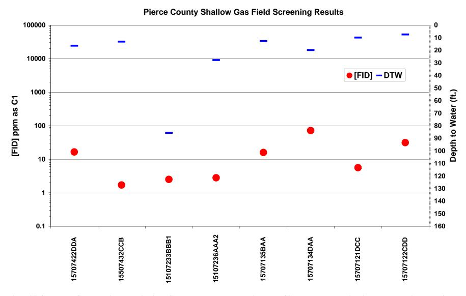
Figure 24. Shallow gas field screening results in Pierce County. FID response [FID] in ppm as C1 plotted on the logarithmic scale on the primary y-axis. Depth to water measurements are plotted on the secondary y-axis.
