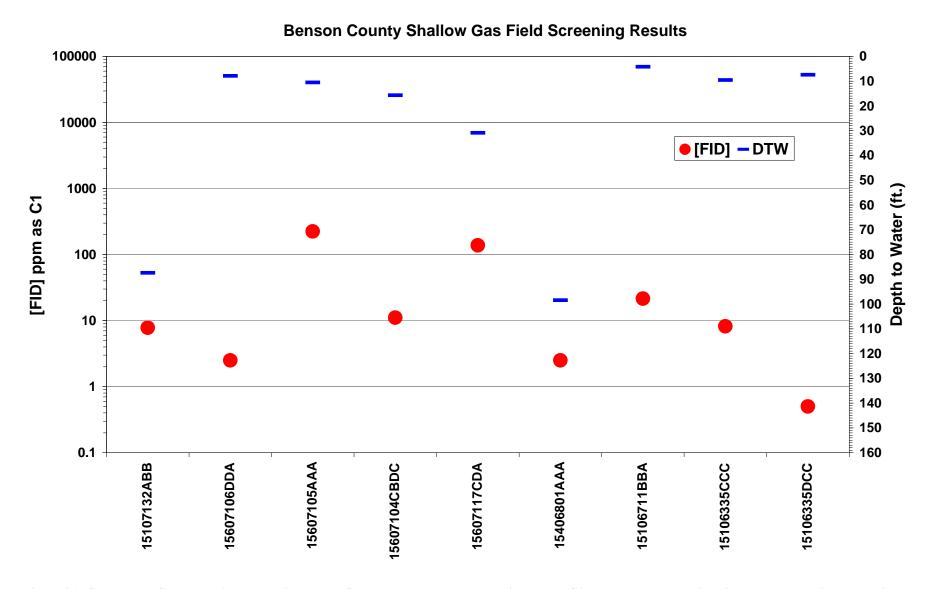
Figure 26. Shallow gas field screening results in Benson County. FID response [FID] in ppm as C1 plotted on the logarithmic scale on the primary y-axis. Depth to water measurements are plotted on the secondary y-axis.
