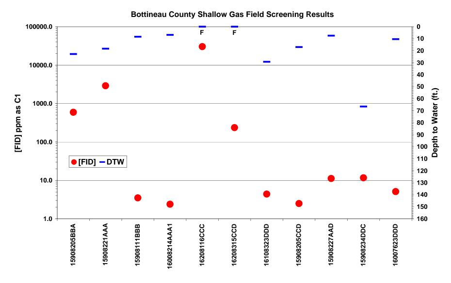
Figure 11. Shallow gas field screening results in Bottineau County. FID response [FID] in ppm as C1 plotted on the logarithmic scale on the primary y-axis. Depth to water measurements are plotted on the secondary y-axis. Flowing wells (F) are highlighted.
