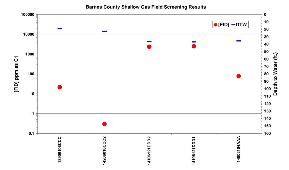
Figure 21. Shallow gas field screening results in Barnes County. FID response [FID] in ppm as C1 plotted on the logarithmic scale on the primary y-axis. Depth to water measurements are plotted on the secondary y-axis. Well with no measurable water level (D) highlighted.
