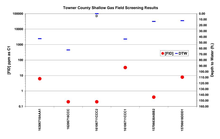
Figure 16. Shallow gas field screening results in Towner County. FID response [FID] in ppm as C1 plotted on the logarithmic scale on the primary y-axis. Depth to water measurements are plotted on the secondary y-axis. Well with no measurable water level (D) highlighted.
