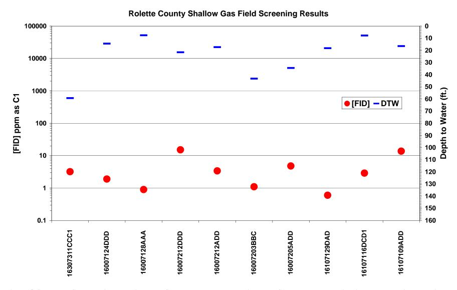
Figure 15. Shallow gas field screening results in Rolette County. FID response [FID] in ppm as C1 plotted on the logarithmic scale on the primary y-axis. Depth to water measurements are plotted on the secondary y-axis.
