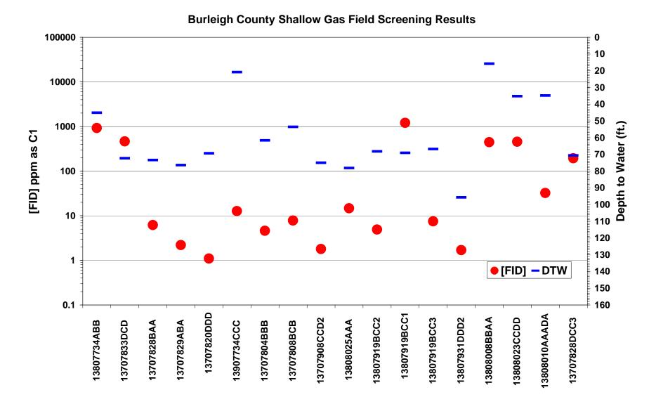
Figure 17. Shallow gas field screening results in Burleigh County. FID response [FID] in ppm as C1 plotted on the logarithmic scale on the primary y-axis. Depth to water measurements are plotted on the secondary y-axis.
