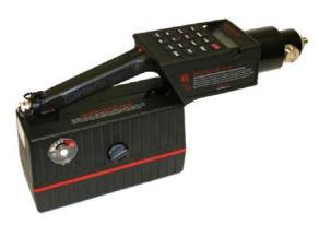
Figure 2. Photovac portable Flame Ionization Detector (FID) used in this investigation.
