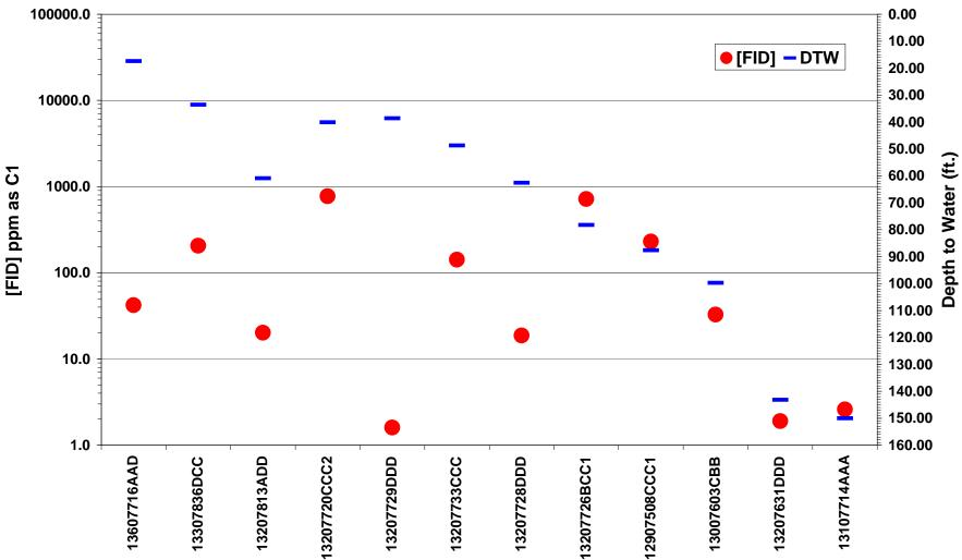
Figure 13. Shallow gas field screening results in Emmons County. FID response [FID] in ppm as C1 plotted on the logarithmic scale on the primary y-axis. Depth to water measurements are plotted on the secondary y-axis.
