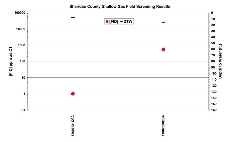
Figure 25. Shallow gas field screening results in Sheridan County. FID response [FID] in ppm as C1 plotted on the logarithmic scale on the primary y-axis. Depth to water measurements are plotted on the secondary y-axis.
