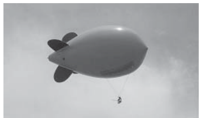
Figure 2. Helium blimp in flight with camera rig suspended underneath. The blimp measures 13 feet (4 m) long and can lift up to 5 pounds payload.
