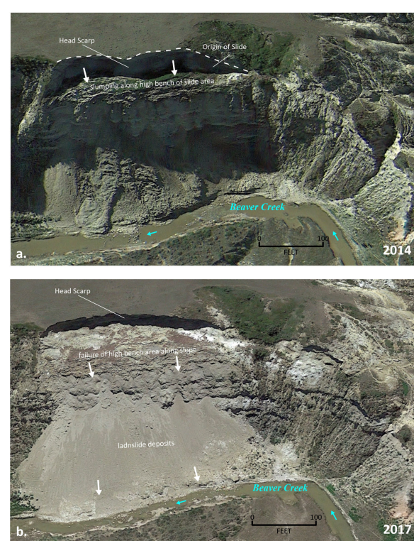
Figure 3. Example of a bedrock landslide in northeastern Golden Valley County along Beaver Creek (view is to the south). This landslide began in the western portion of the slide area ca. 2000 and progressed eastward with the failure of the upper scarp along a high bench within the slide area (a) prior to 2014. The upper bench continued to slump (b), covering the lower portion of the slide area with landslide deposits intruding into the channel of the creek in 2017. This landslide area remains active.
