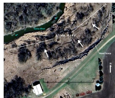
Figure 3. Example of riverbank slumping in central Trail County along the Goose River one mile southeast of the Norway bridge and seven miles west of Mayville. A well developed head scarp is visible near the property access road.
