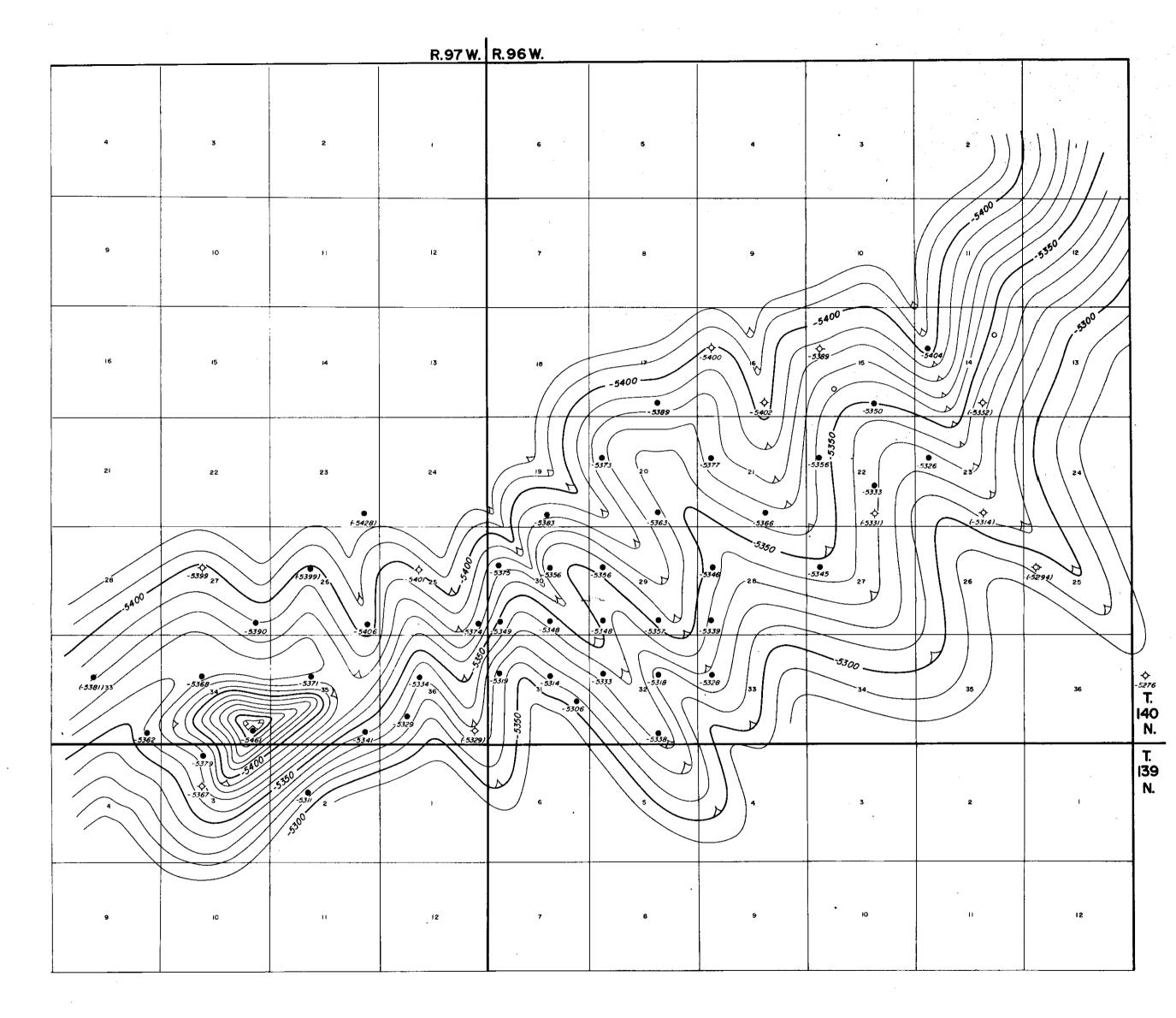
DICKINSON-WEST DICKINSON FIELDS STARK COUNTY, NORTH DAKOTA STRUCTURE CONTOUR MAP TOP OF THE HEATH "B" SAND POROSITY (OR ITS STRATIGRAPHIC EQUIVALENT IN NON-POROUS WELLS) CONTOUR INTERVAL = 10'
