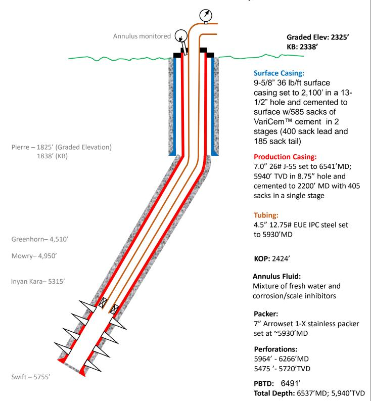
\*\*\*\* Not to scale. All depths referenced from estimated KB elevation of 2338' and calculated from NDIC's call of geologic tops in the offsetting RAVIN 26-35-2H (WF# 21994)
