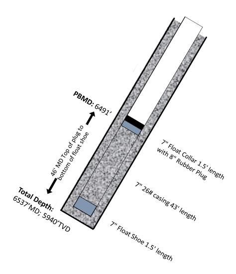
\*\*\*\* Not to scale. All depths referenced from estimated KB elevation of 2338' and calculated from NDIC's call of geologic tops in the offsetting RAVIN 26-35-2H (WF# 21994)
