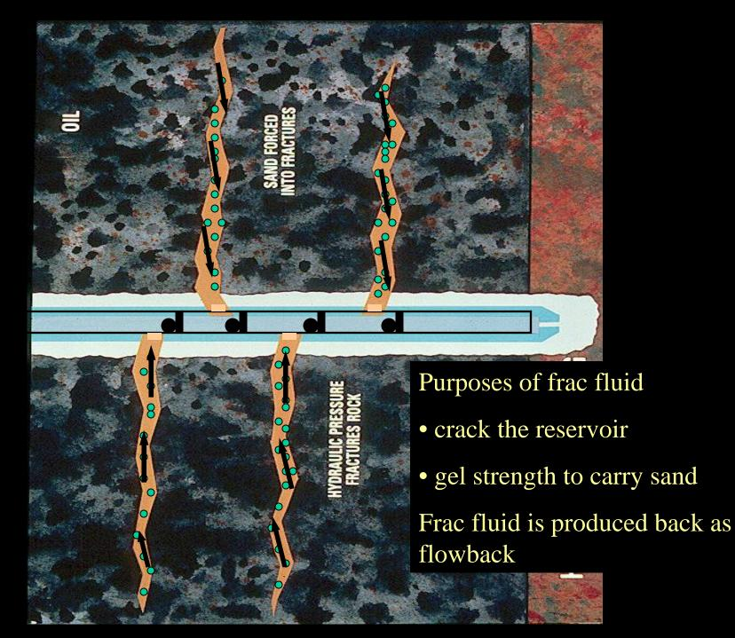
**Hydraulic Fracturing:** Mixture of water, sand and chemicals pressurized and pumped into the well to form microscopic fractures in shale.
